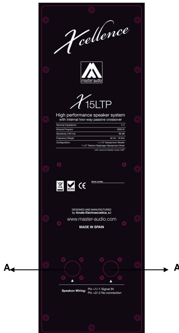
Fig.2. X15LTP connection panel
